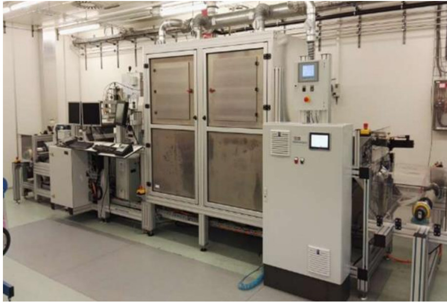
Figure 5. Middle part of the line with the curing box of of the pilot plant.
