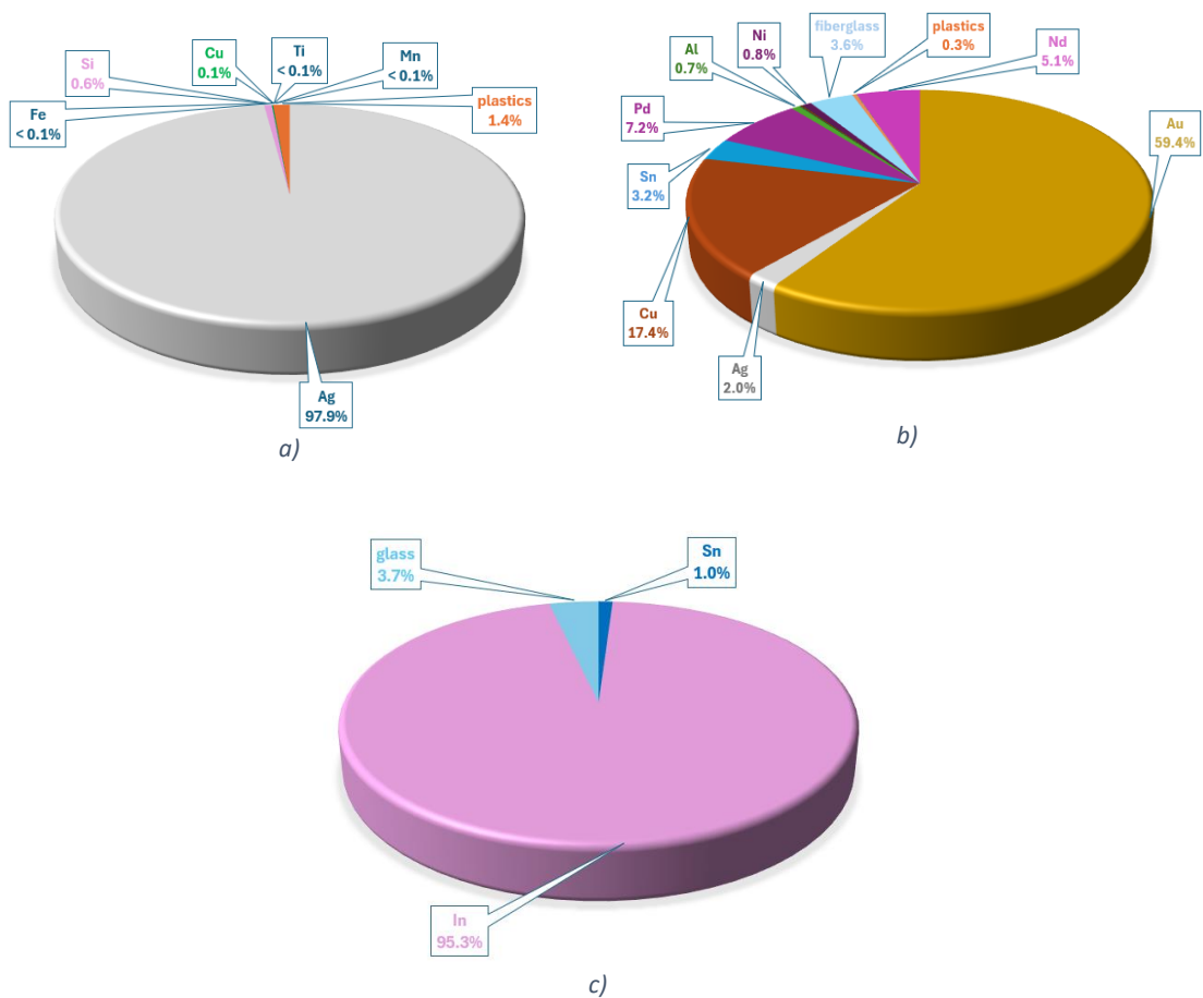
Figure 17. Incidence of the different elements on the overall IEV. a) IME; b) PCBs of combi-meter; c) ITO glass of LCDs
