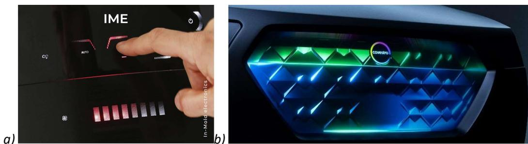
Figure 1a) climate control unit by WalterPack; b) Automotive front grill demonstrator by Covestro: 5D film insert molding (FIM) combines rear 3D structures with color and decoration due to the design freedom enabled by printed polycarbonate films. Integrated metal lines can be used for example for deicing to keep sensor areas clear or provide brand differentiation through integrated LED lighting powered by printed electronics.
