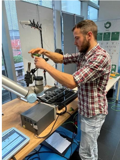
Figure 21. Pollini's operator performing a manual tool change operation equipping the robot with a two-finger electric gripper.
