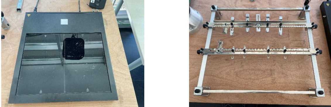
Figure 5 – The preheating plate and the modified frame
