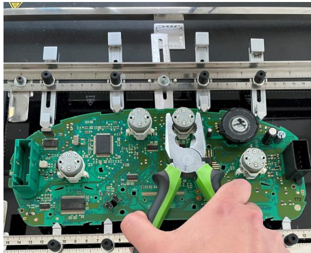
Figure 18. Removal of TH components
