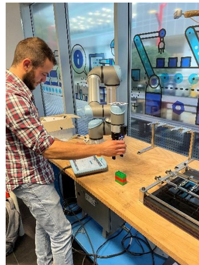
Figure 23. Pollini's operator testing the cobot and the pilot plant for semi-automated PCB disassembly.
