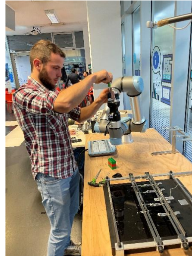
Figure 21. Pollini's operator performing a manual tool change operation equipping the robot with a two-finger electric gripper.
