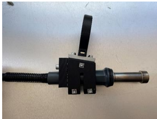
Figure 4 – The custom holder for the air-desolderer
