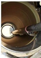
Figure 14: Squeegee inside the rotary screen.
